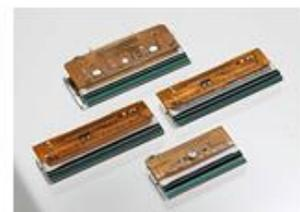
Kyocera's Thermal Printheads for FAX (left) and Card Printers (right)
